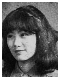
Fig. 9. Printing plate (200 lpi) obtained from the system EPP/NIOTf with P-8003 binder polymer. Experimental condition: exposure energy = 0.5 mJ/cm 2 ; PEB 2 min.
